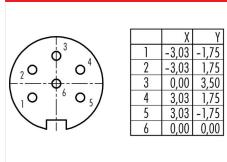
Contact arrangement (Plug-in side)
